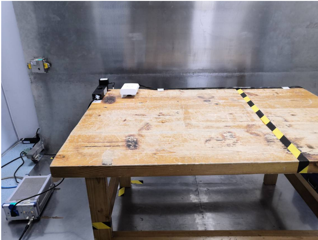
Conducted Emissions Side View-Adapter Power Mode
