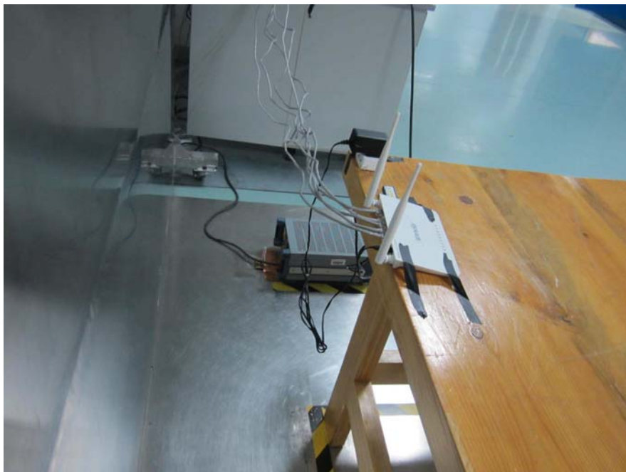
Conducted Emissions – Rear View
