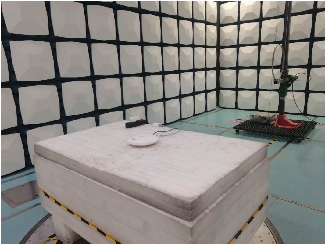
Radiated Emission 9k-30MHz Perpendicular View
