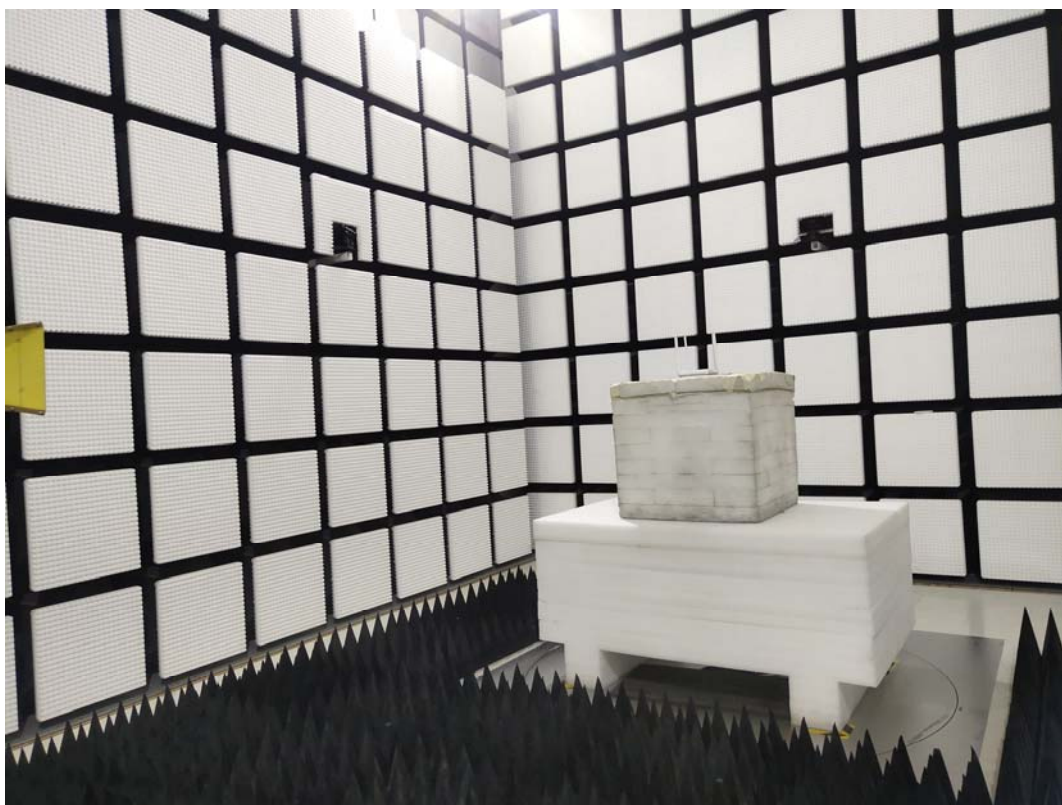
Radiated Emission Above 1GHz View
