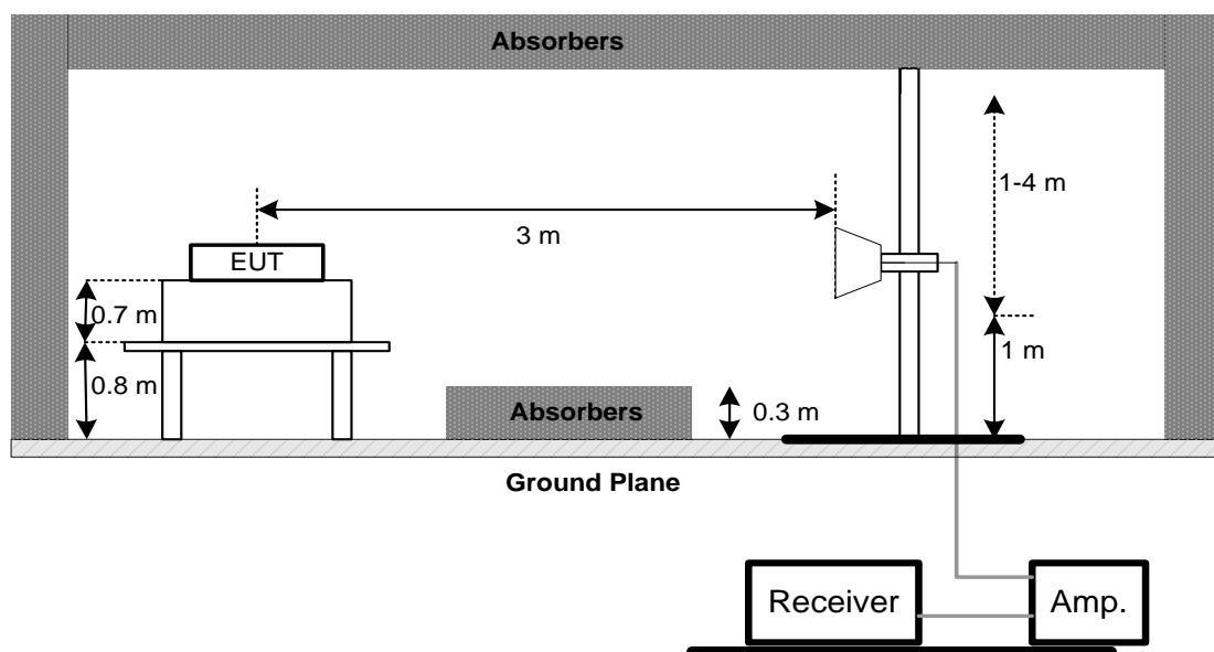
(C) For Radiated Emissions Below 30MHz
