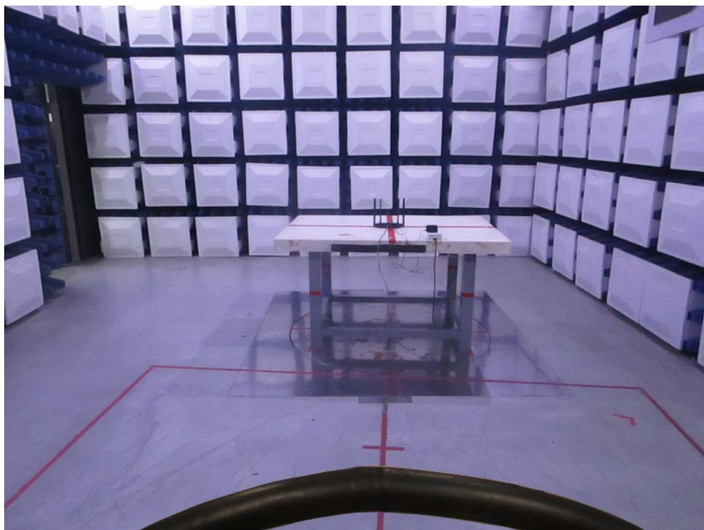
**Radiated Emissions Test Photos****30 MHz to 1 GHz**
