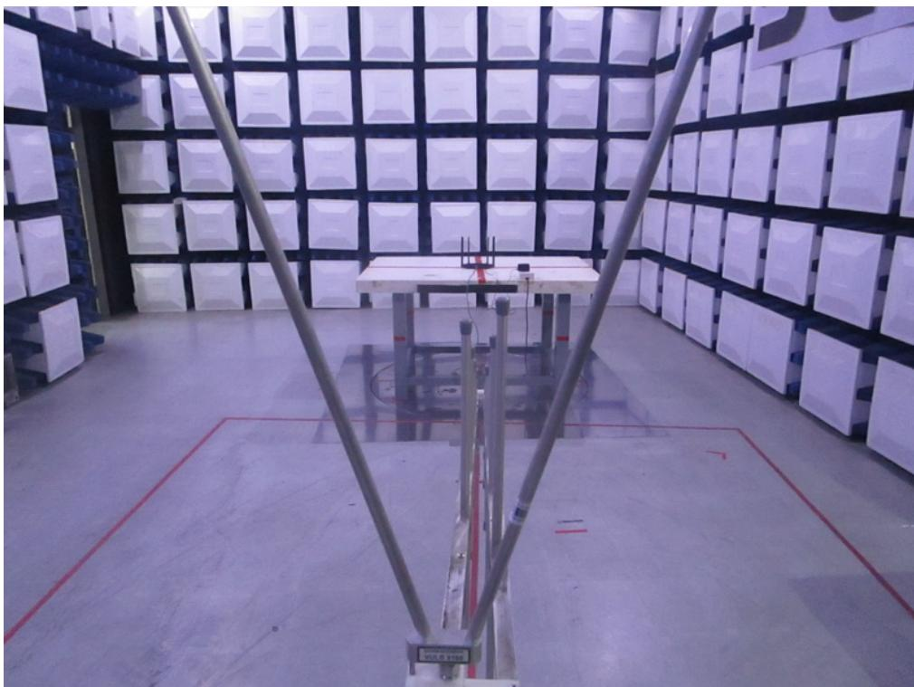
**Radiated Emissions Test Photos****Above 1 GHz**
