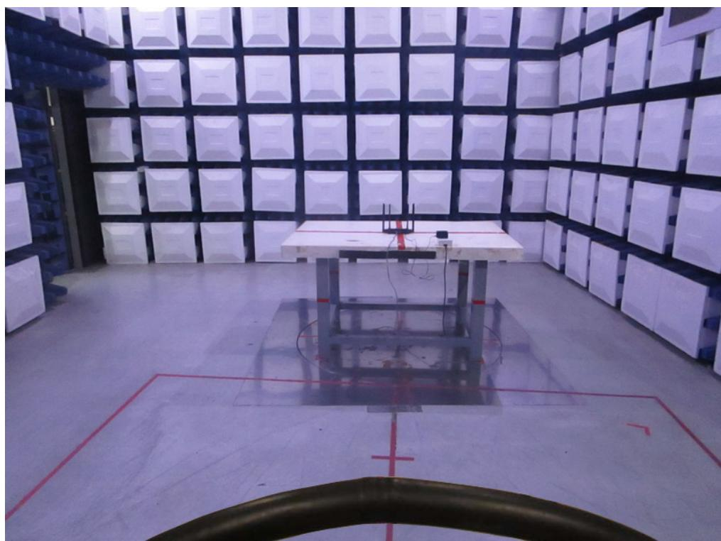
**Radiated Emissions Test Photos****30 MHz to 1 GHz**
