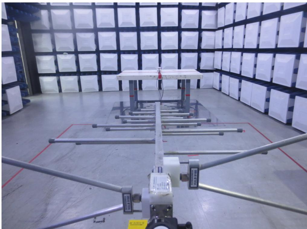
**Radiated Emissions Test Photos****Above 1 GHz**
