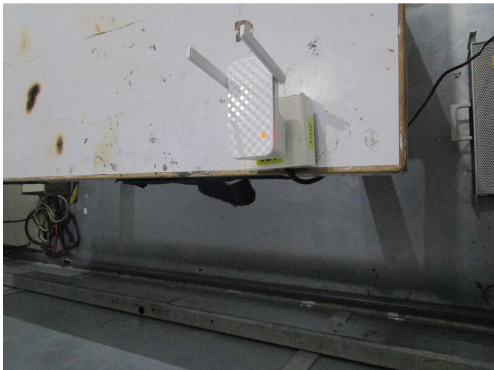
**Radiated Emissions Test Photos****9 kHz to 30 MHz**
