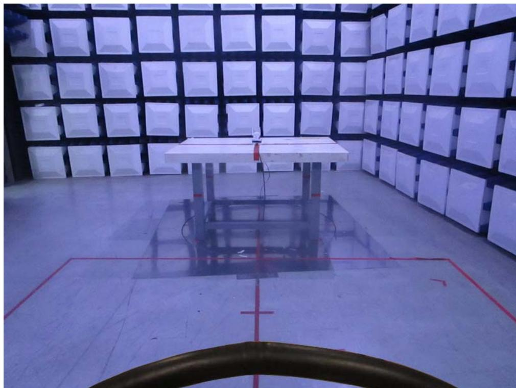
**Radiated Emissions Test Photos****30 MHz to 1 GHz**
