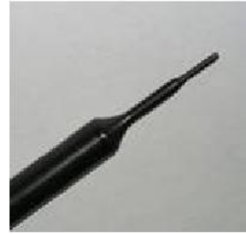
Figure 4.4 EX3DV4 E-field Probe
