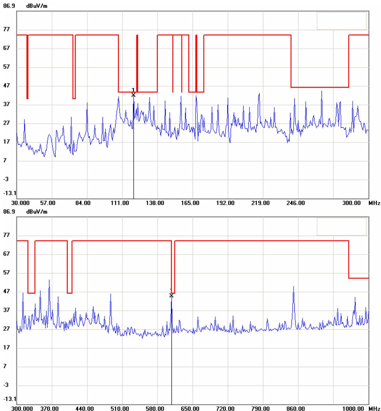
1. The attached measurement plots are preliminarily pre-scanned with peak detector for determining the final checking frequencies and are for reference only.
