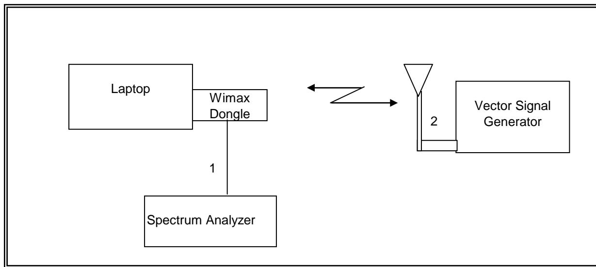
**SETUP DIAGRAM FOR RADIATED TESTS**
