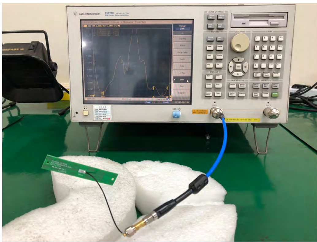
Figure 2: Testing with network analyzer
