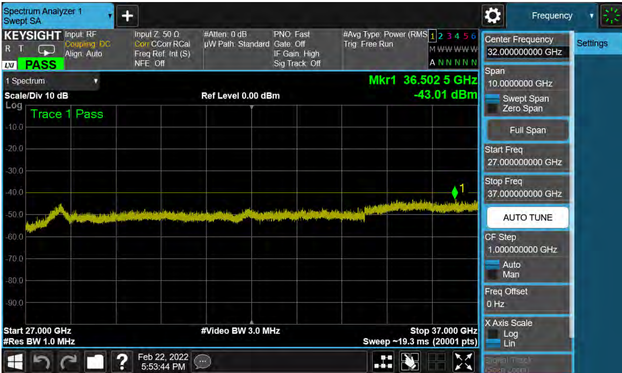
Plot 8-40. Conducted Spurious Plot (ULCA LTE Band 48 – 20+20MHz QPSK – High Channel)
