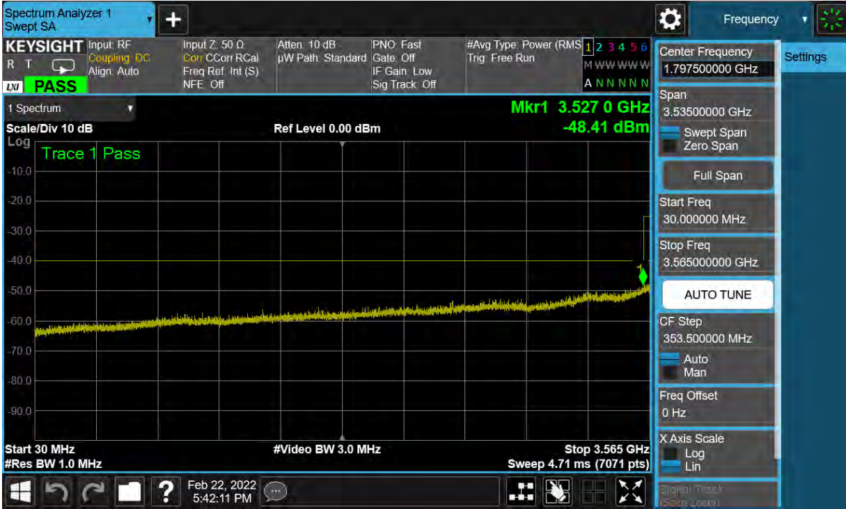
Plot 8-33. Conducted Spurious Plot (ULCA LTE Band 48 – 20+20MHz QPSK – Mid Channel)
