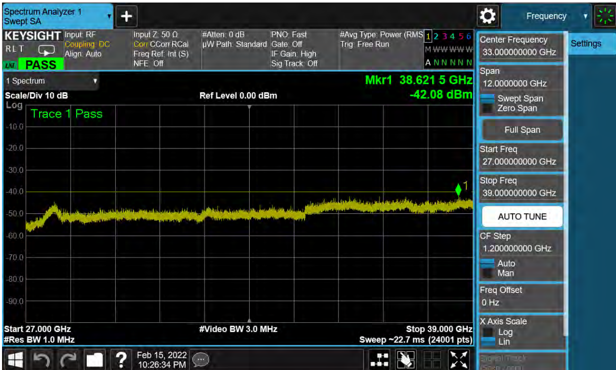
Plot 8-28. Conducted Spurious Plot (LTE Band 48 - 5MHz 16QAM - RB Size 1, RB offset 12 - High Channel)
