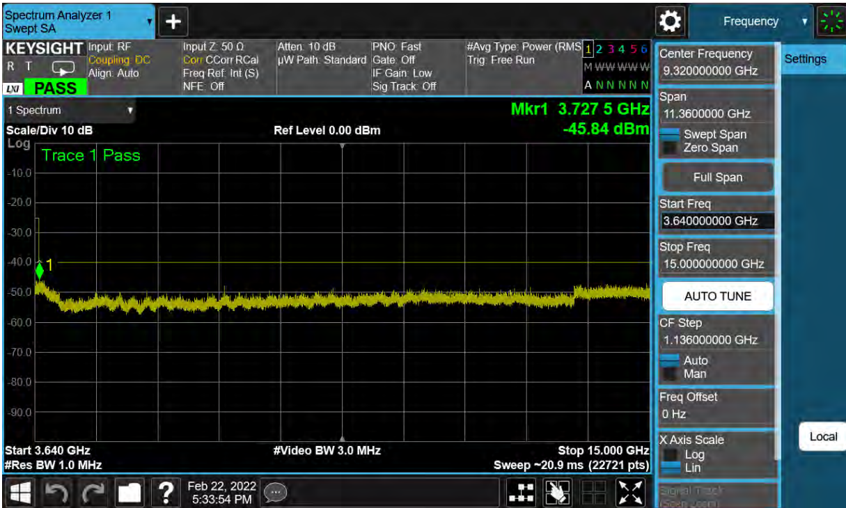
Plot 8-30. Conducted Spurious Plot (ULCA LTE Band 48 – 20+20MHz QPSK – Low Channel)
