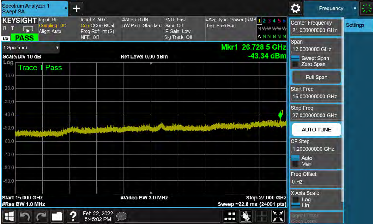
Plot 8-35. Conducted Spurious Plot (ULCA LTE Band 48 – 20+20MHz QPSK – Mid Channel)
