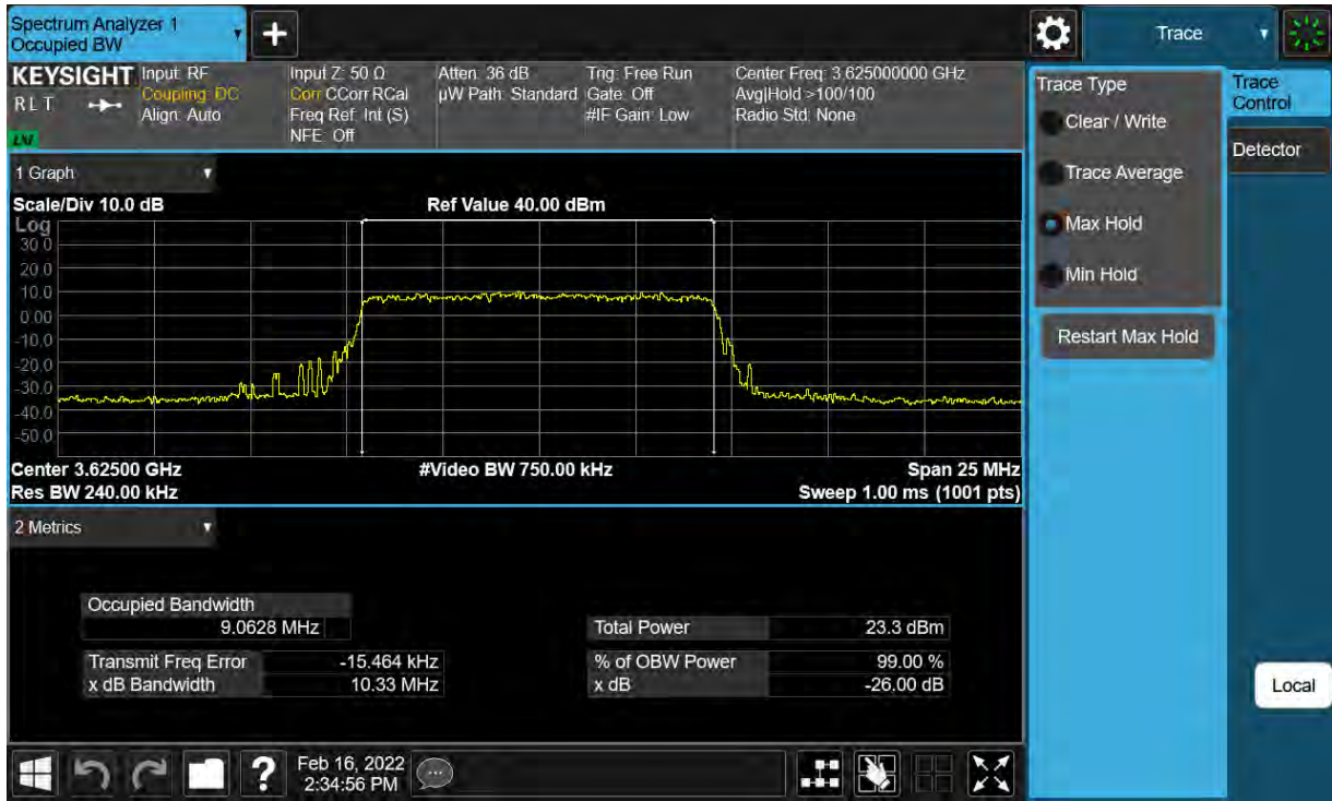
Plot 8-3. Occupied Bandwidth Plot (LTE Band 48 – 10MHz QPSK – Full RB Configuration)
