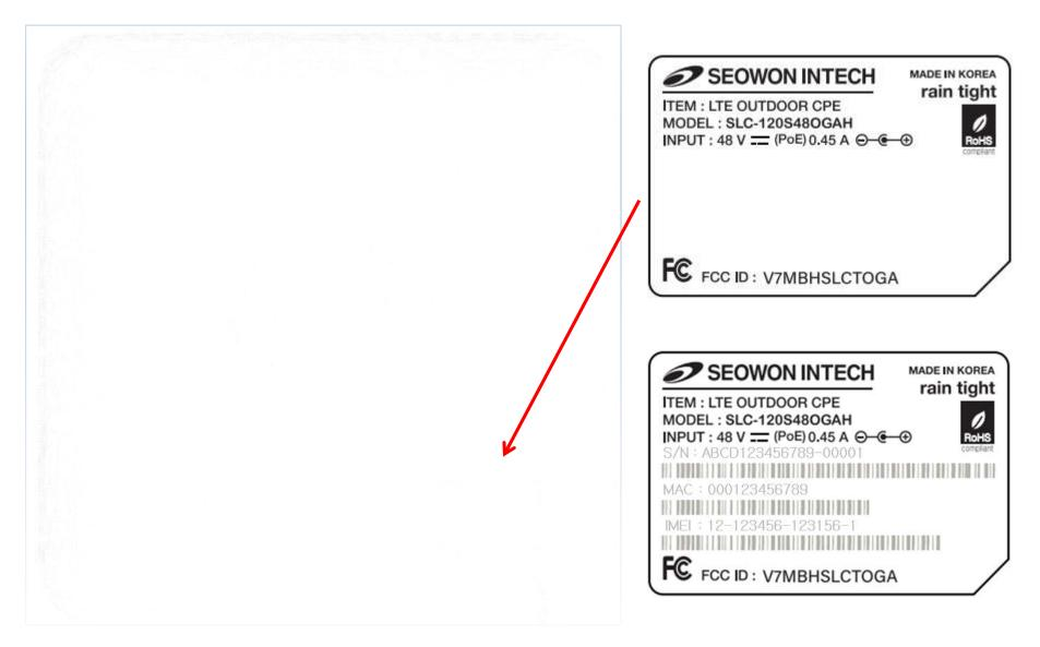
White PP Film + AT20 Adhesive label paper + Label printed with UV BLACK ink is attached to the embossed position.
