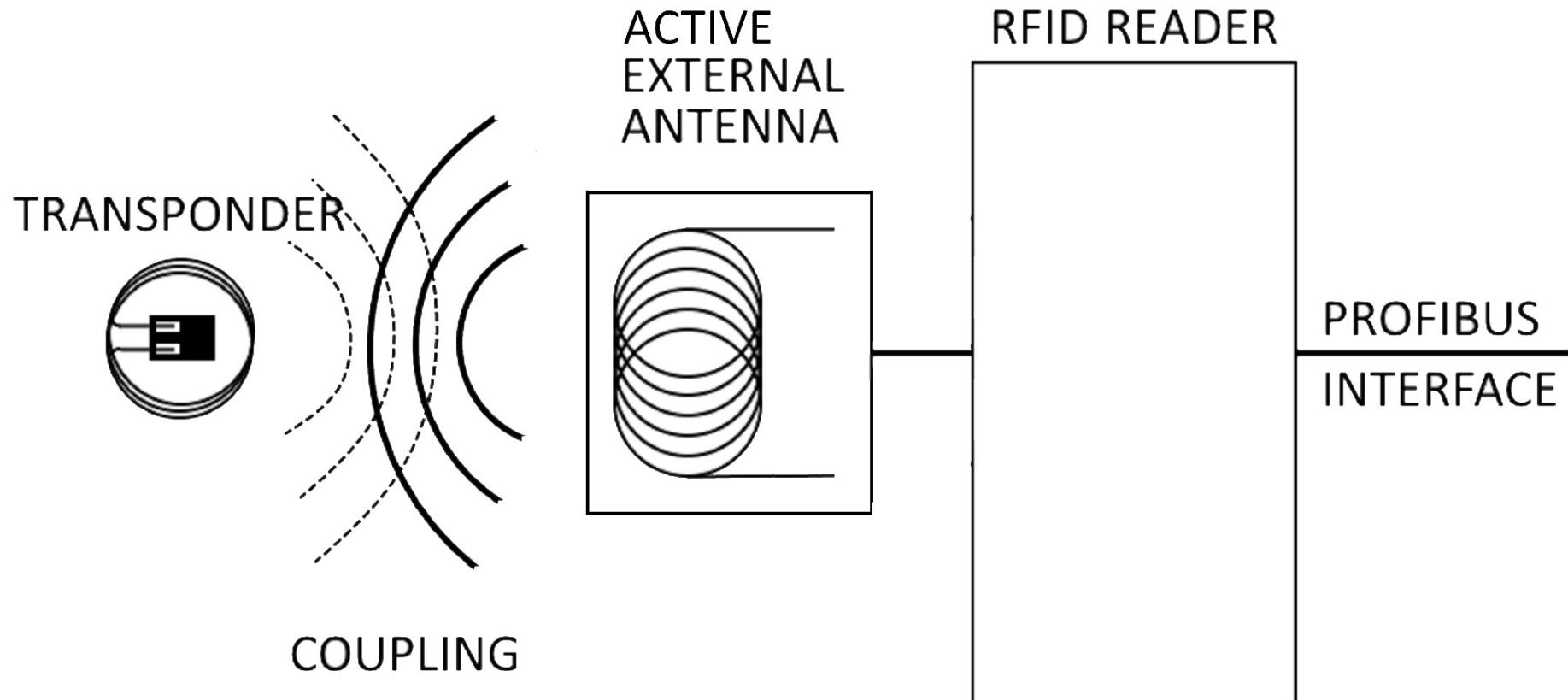
For reading a passive transponder, the RFID reader is generating an electromagnetic field. This happens when the reader is receiving a command. The electromagnetic field is powering the transponder which is modulating its UID on the exitation field. The reader receives the signal, demodulates the UID and transfers it via Profibus.
