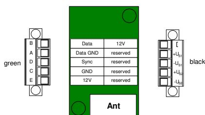
Pin assignment antenna connector:
