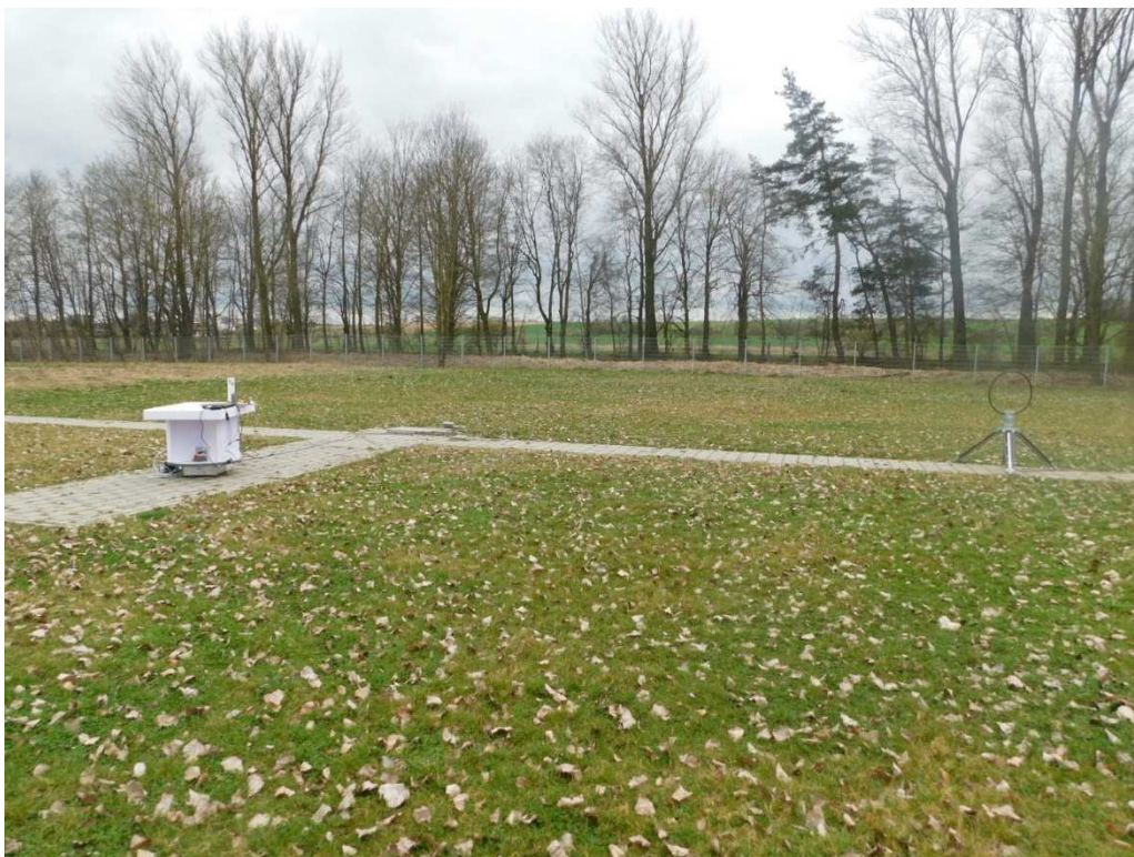
Pre-compliance test setup Test setup 3 m – Antenna orientation vertical / parallel
