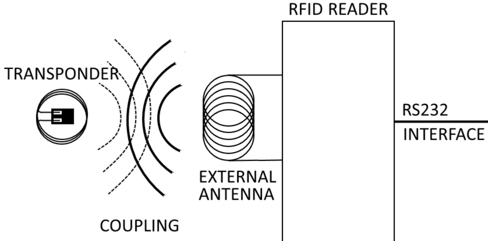
For reading a passive transponder, the RFID reader is generating an electromagnetic field. This happens, depending on the operation mode, permanently or when the reader is receiving a command. The electromagnetic field is powering the transponder which is modulating its UID on the exitation field. The reader receives the signal, demodulates the UID and transfers it via RS232.
