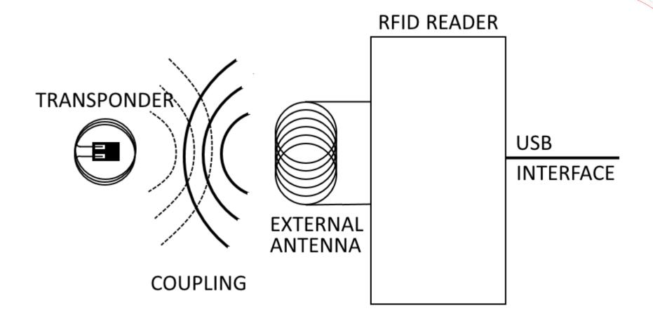
For reading a passive transponder, the RFID reader is generating an electromagnetic field. This happens, depending on the operation mode, permanently or when the reader is receiving a command. The electromagnetic field is powering the transponder which is modulating its UID on the exitation field. The reader receives the signal, demodulates the UID and transfers it via USB.
