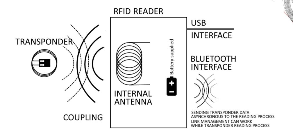
For reading a passive transponder, the RFID reader is generating an electromagnetic field. This happens triggered manualy by pressing a reader button. The electromagnetic field is powering the transponder which is modulating its UID on the exitation field. The reader receives the signal, demodulates the UID and transfers it via USB or Bluetooth.
