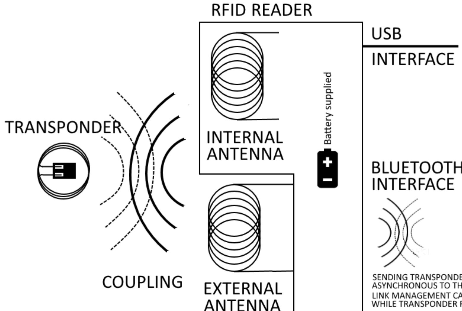
For reading a passive transponder, the RFID reader is generating an electromagnetic field. Only with one antenna. This happens triggered manually by pressing a reader button. The electromagnetic field is powering the transponder which is modulating its UID on the exitation field. The reader receives the signal, demodulates the UID and transfers it via USB or Bluetooth.
