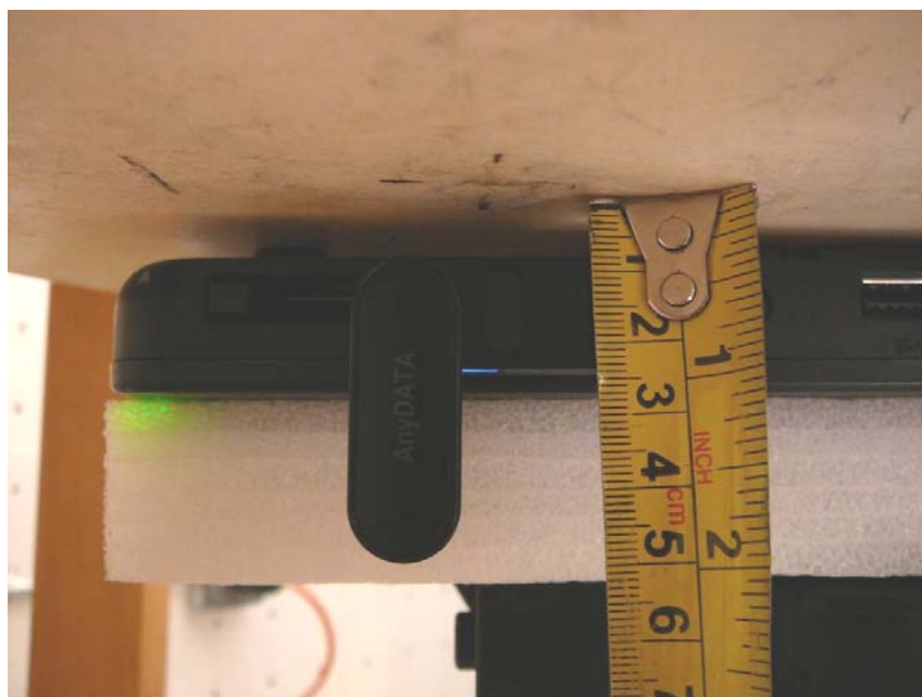
EUT Horizontal-Down with Antenna 90 Degree within 10mm Separation to Flat Phantom with Dell Laptop (Inspiron 1300) Setup Photo
