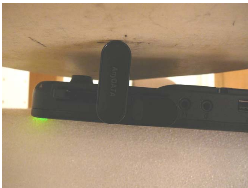
EUT Horizontal-Down with Antenna 270 Degree within 10mm Separation to Flat Phantom with Dell Laptop (Inspiron 1300) Setup Photo
