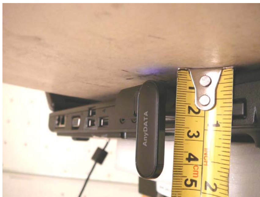
EUT Horizontal-Up with Antenna -90 Degree within 10mm Separation to Flat Phantom with Dell Laptop (Inspiron 1300) Setup Photo
