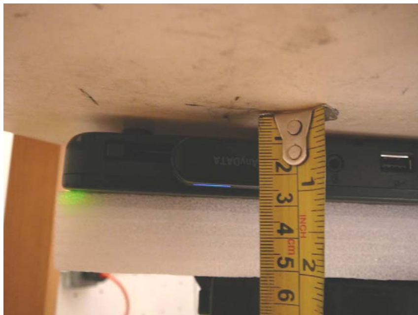
EUT Horizontal-Down with Antenna 0 Degree within 10mm Separation to Flat Phantom with Dell Laptop (Inspiron 1300) Setup Photo
