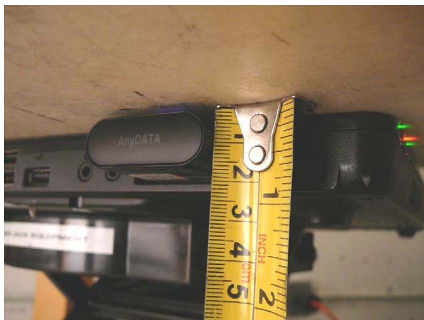
EUT Horizontal-Up with Antenna 0 Degree within 10mm Separation to Flat Phantom with Dell Laptop (Inspiron 1300) Setup Photo
