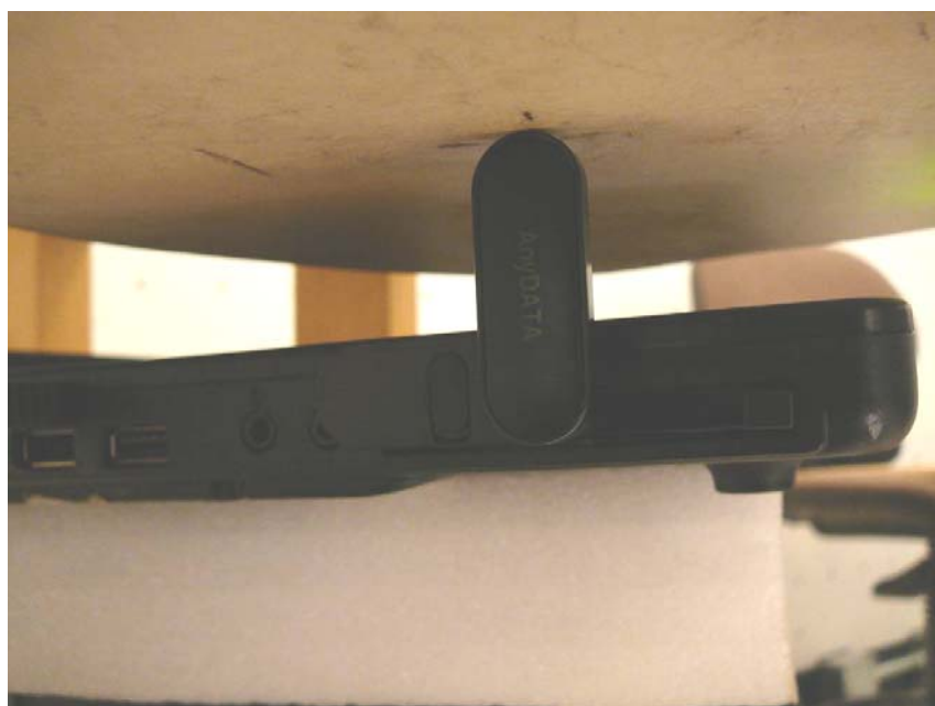
EUT Horizontal-Up with Antenna –270 Degree within 10mm Separation to Flat Phantom with Dell Laptop (Inspiron 1300) Setup Photo
