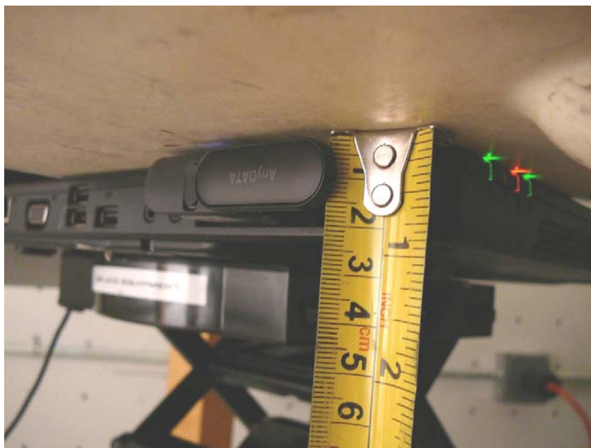
EUT Horizontal-Up with Antenna –270 Degree within 10mm Separation to Flat Phantom with Dell Laptop (Inspiron 1300) Setup Photo
