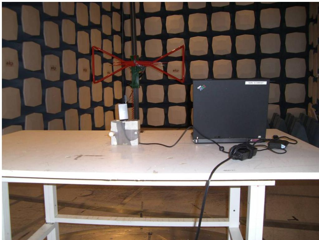
**Radiated Emissions – Front View**
