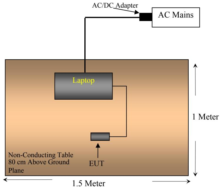
**Test setup Block Diagram for Spurious Radiated Emissions tests**
