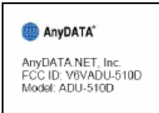
**Specifications:** Text is black or white in color and is left justified. Labels are silk-screened and shall be “permanently affixed” at a conspicuous location on the EUT.
