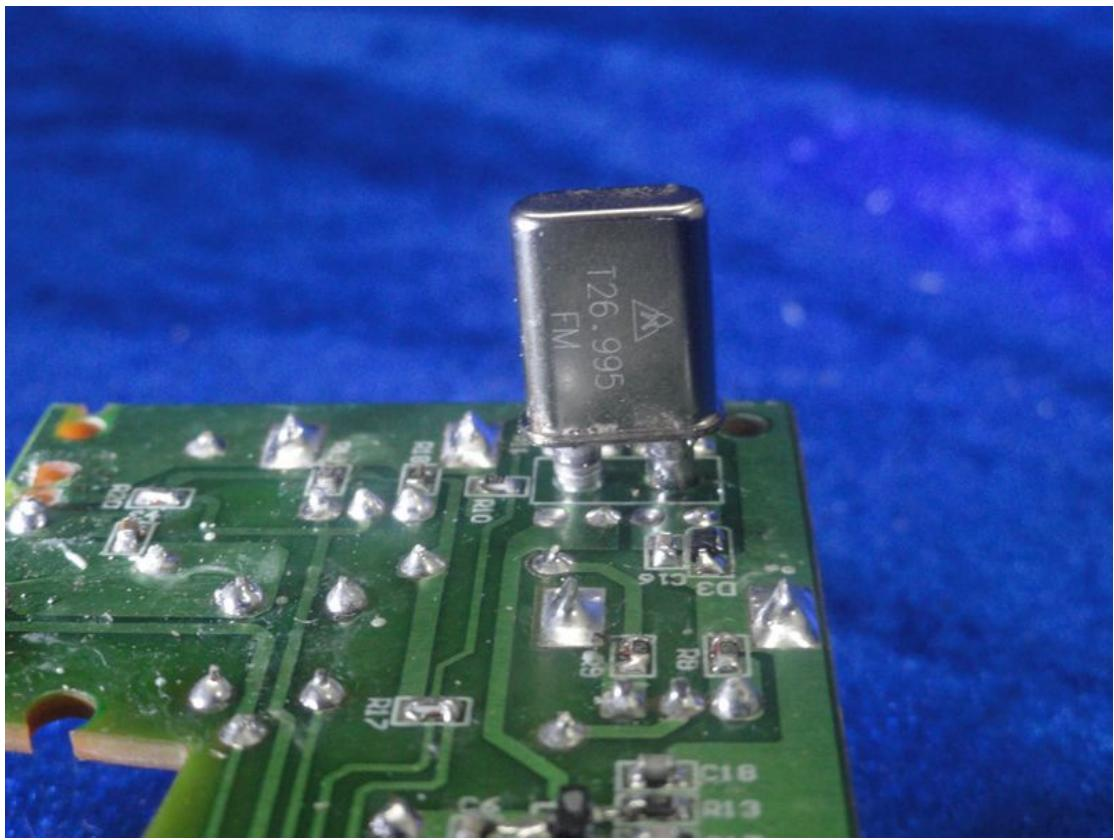
Note: The Crystal is soldered on the PWB
