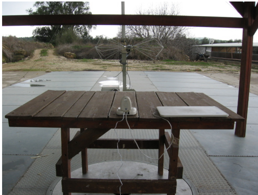
Figure 6. Radiated Emission Test
