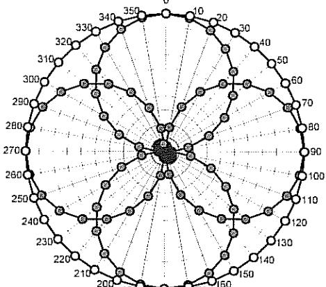
Receiving Pattern ( $\phi$ ),  $\theta = 90^\circ$  $f = 600 \text{ MHz, TEM ifi110EXX}$
