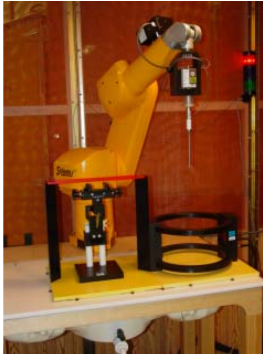
Figure 4.2a T-Coil setup with Helmholtz Coil
