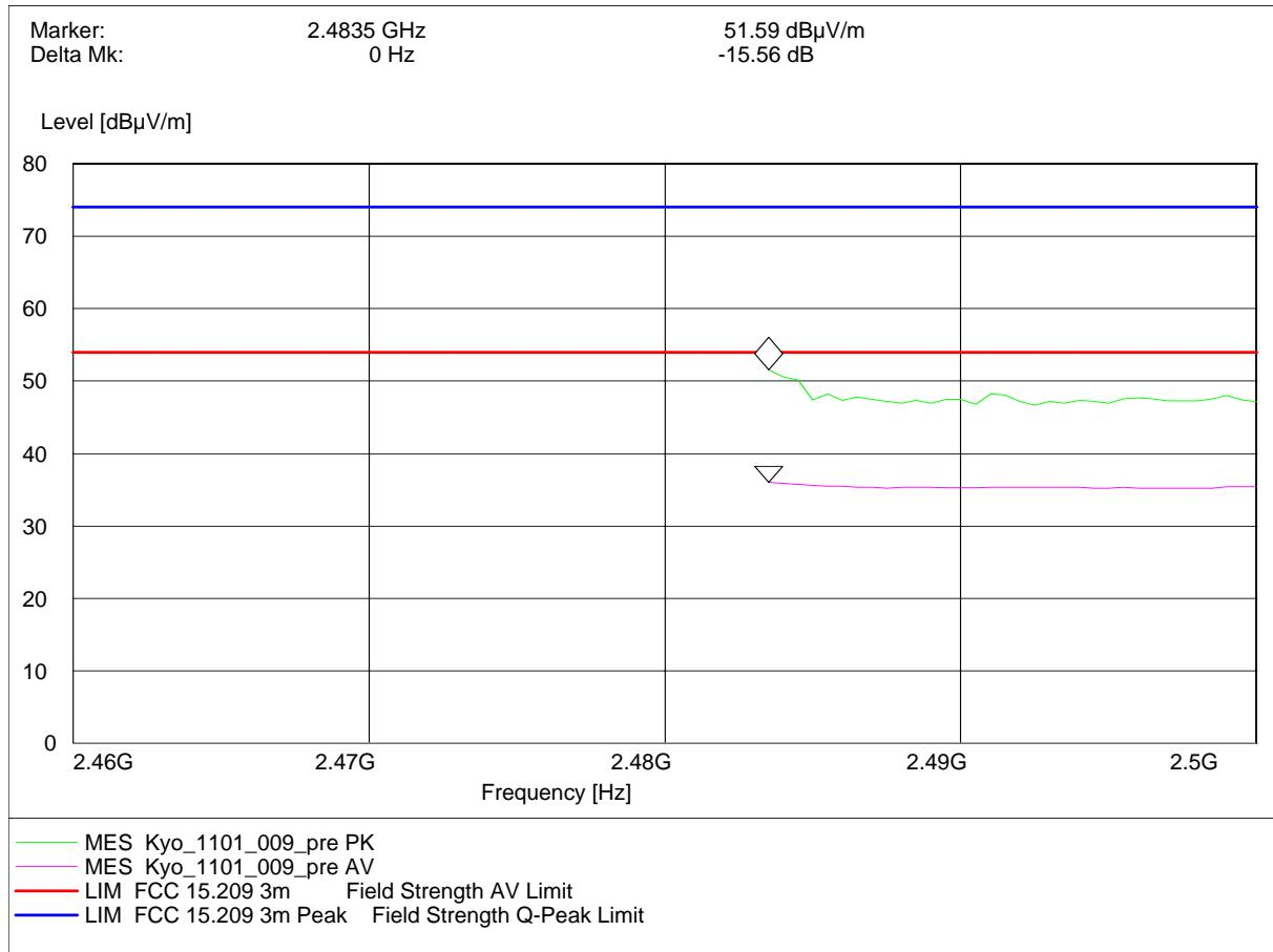
Radiated measurement (higher band edge)
