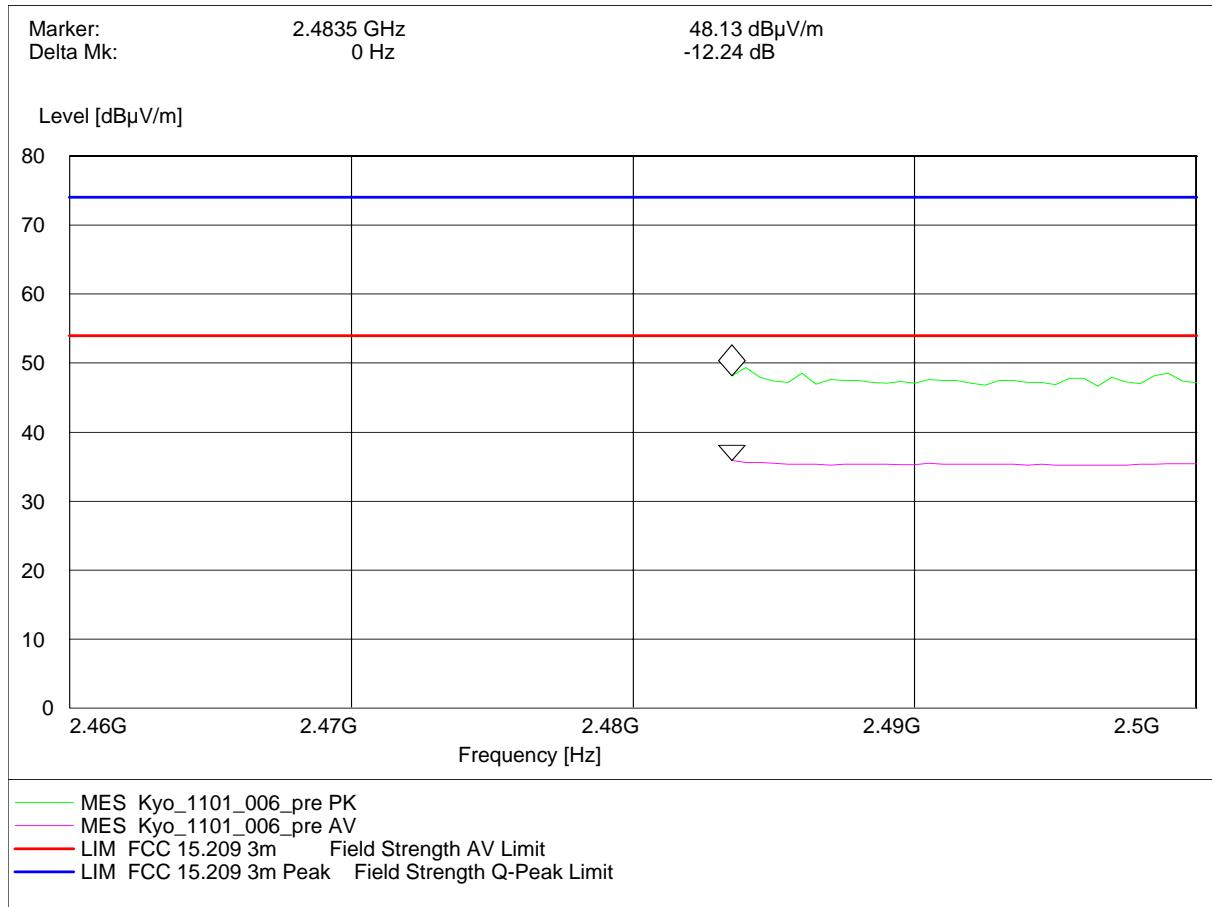
Radiated measurement (higher band edge)
