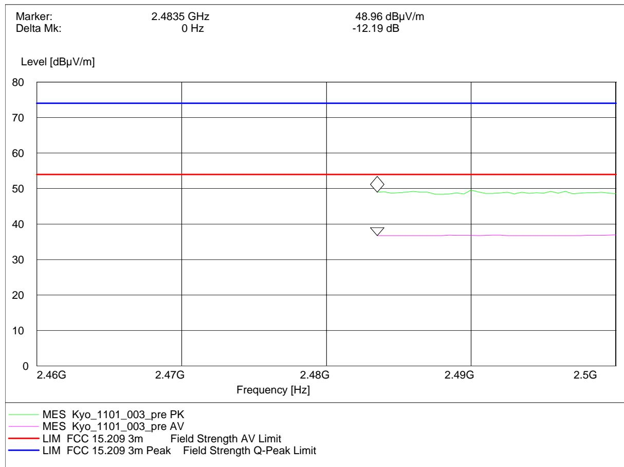
Radiated measurement (higher band edge)
