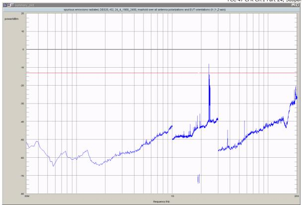
Test3: 24.4; Frequency Band = 1900, Mode = GSM, Channel = 661, Frequency = 1880.0MHz
