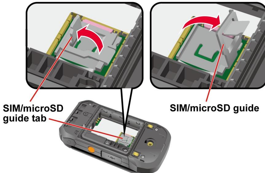
3. Slide the microSD card into the slot with the gold contacts facing down. Gently push the card in until it fits into place.
