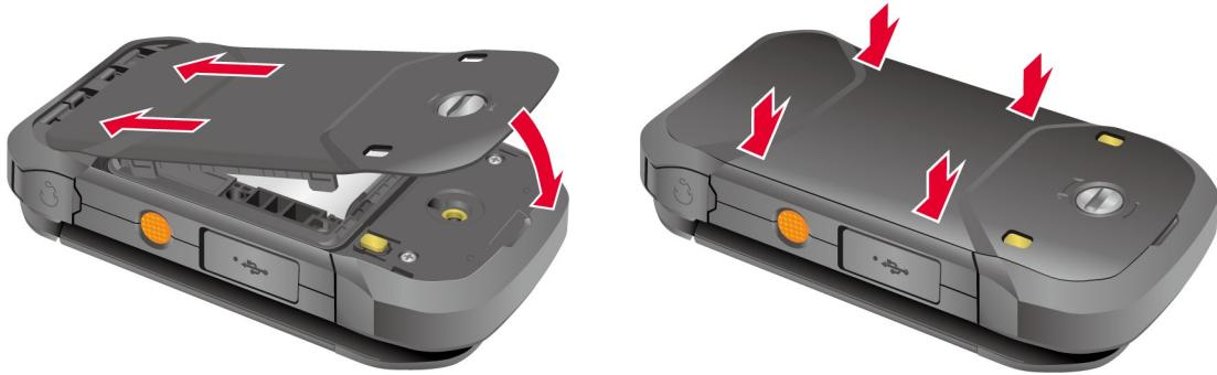
**Warning:** Make sure you press all around the edges of the battery cover to ensure your phone's waterproof seal is intact.
