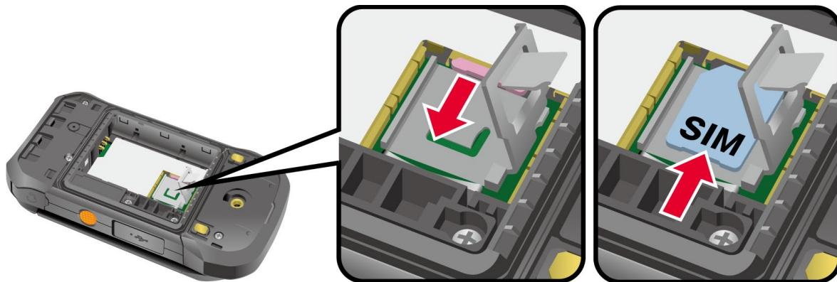
**Note:** Please be careful to not insert the SIM card into the SD card slot.
