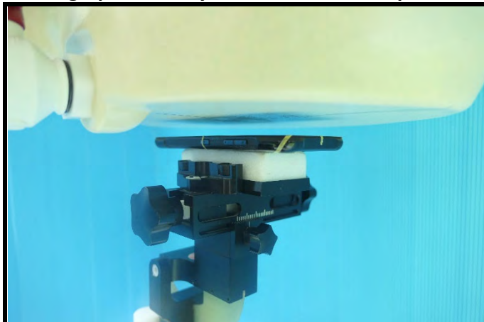
Front Face of EUT Tested at 15 mm
