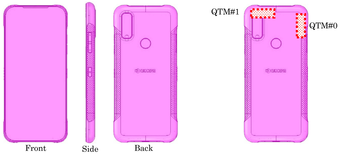
Figure 1. HFSS simulation model which is mounted two mmWave antenna modules.
