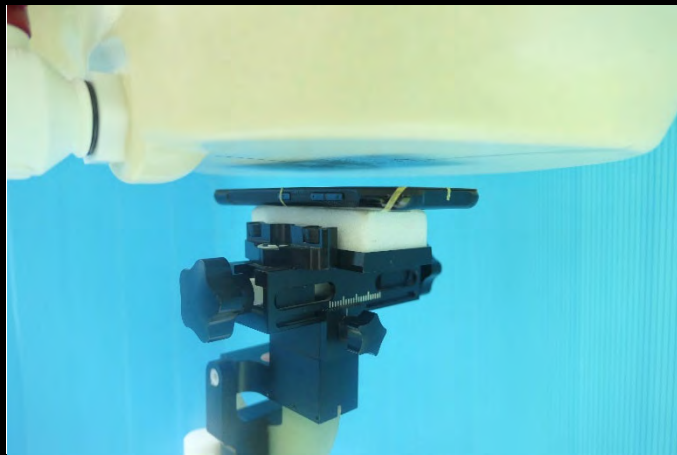
Front Face of EUT Tested at 15 mm
