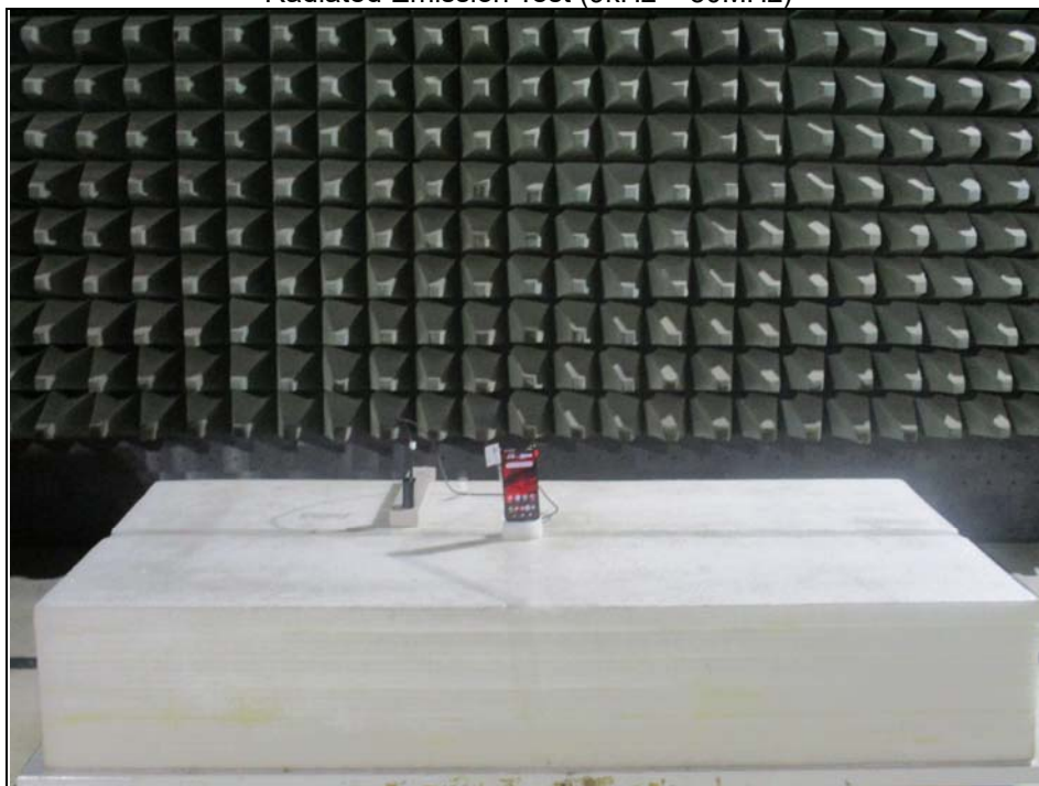
Radiated Emission Test (9kHz ~ 30MHz)
