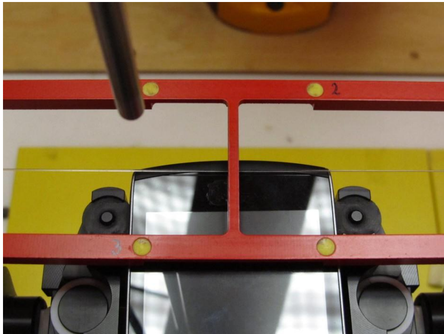
Figure 1b – HAC T-Coil Test Setup
