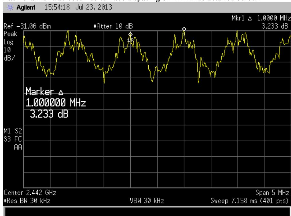
The -20 dB bandwidth for the device has been determined below
