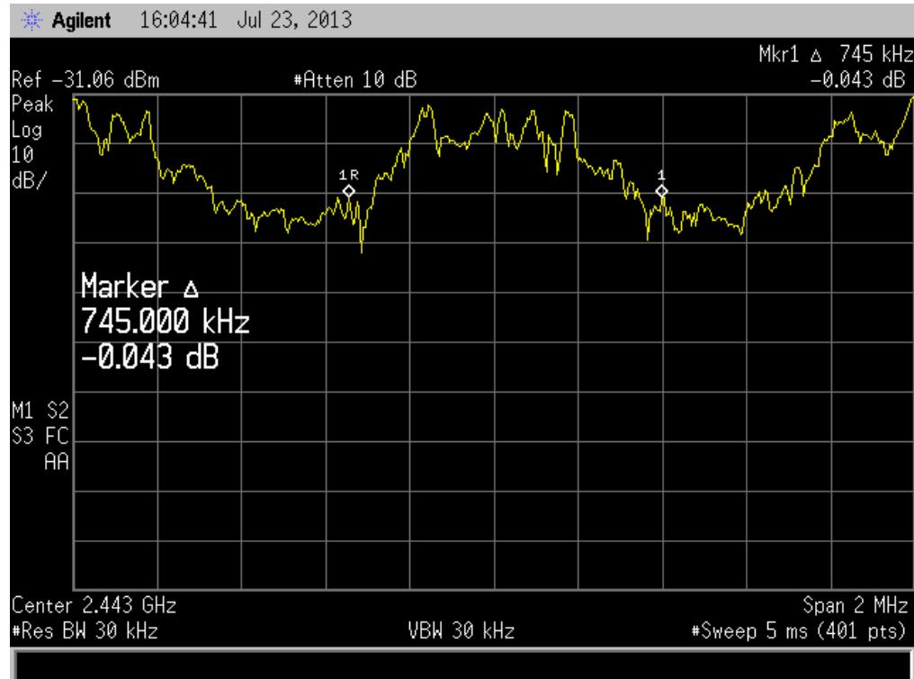
The 20 dB bandwidth is therefore less than the 1 MHz channel spacing.
