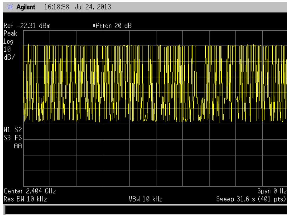
Several tests were then carried out using a 10 second measurement period with the maximum number of transmissions being used to determine the number of transmissions in 31.6 seconds.
