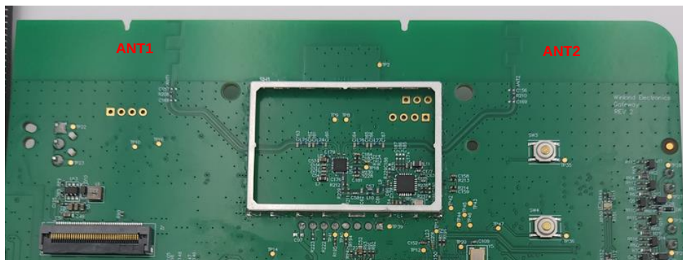
Figure 1: Gateway PCB Antenna Locations
