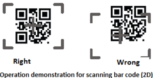
Right,Wrong,Operation demonstration for scanning bar code(2D)
