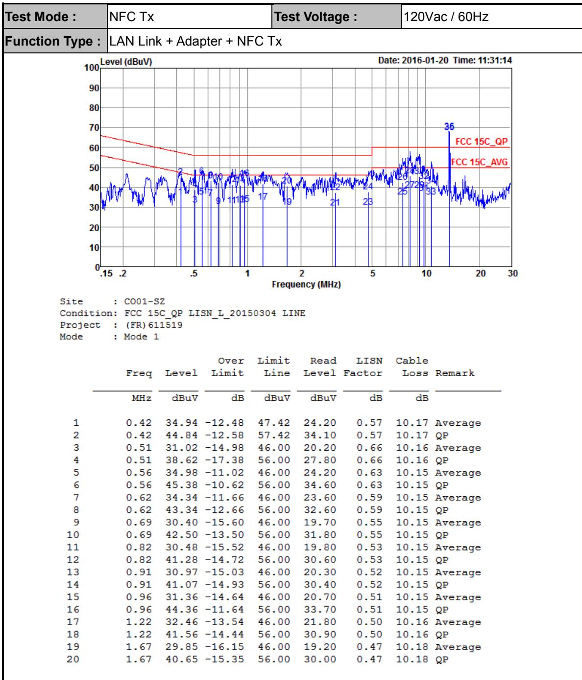
(1) The EUT is with NFC antenna during testing.
