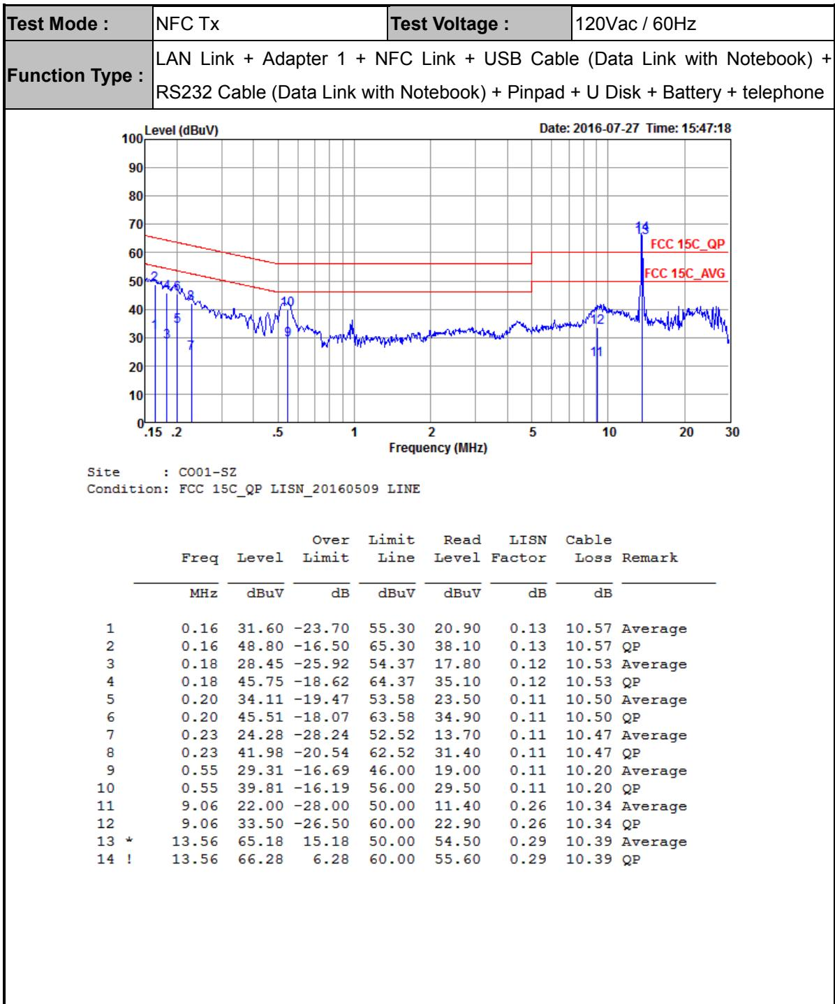
(1) The EUT is with NFC antenna during testing.
