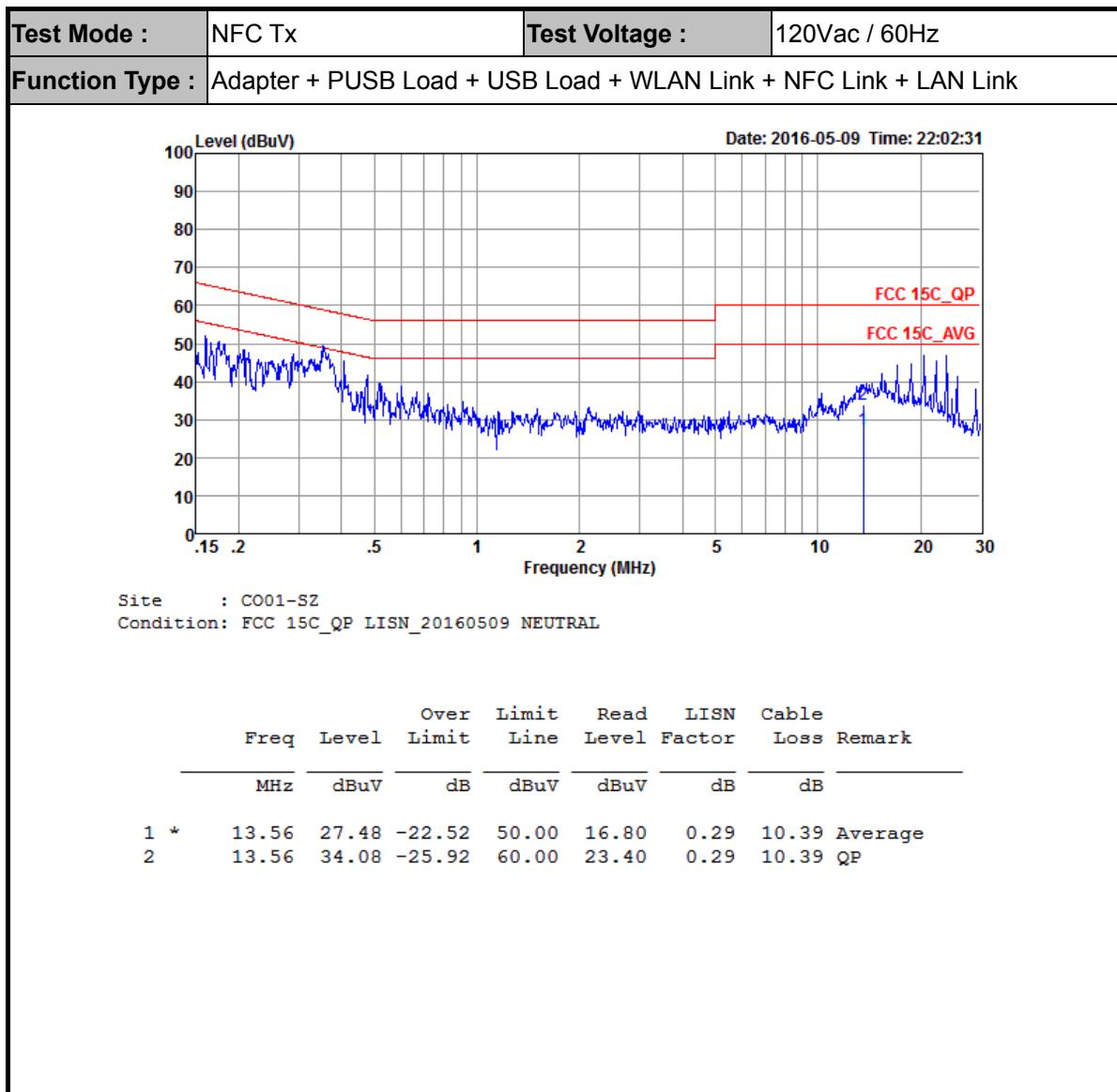
(2) The NFC antenna is replaced by a dummy load during test.
