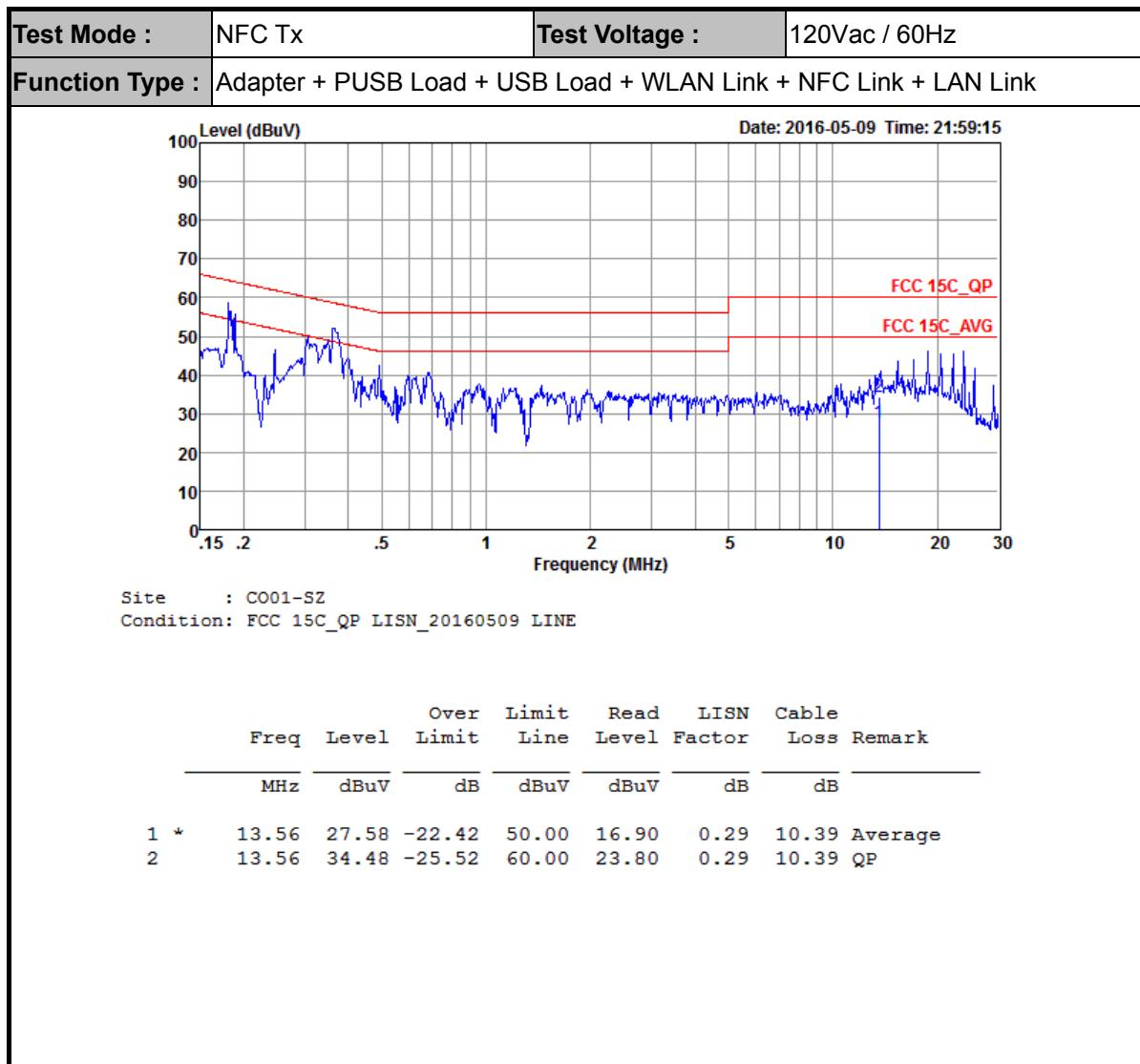
(2) The NFC antenna is replaced by a dummy load during test.
