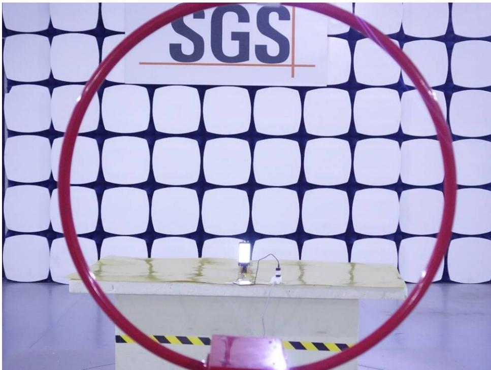
**Radiated Emissions (30MHz-1GHz)**
