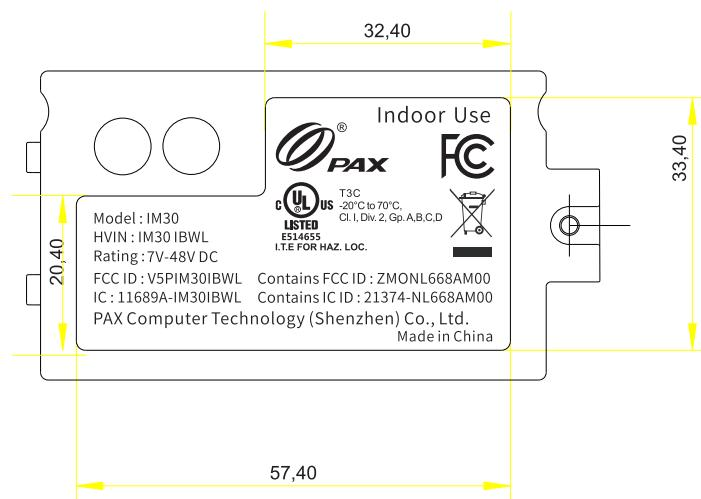
The label is laser-engraved onto the bottom of the product.
