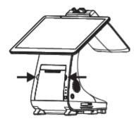
2. Open the built-in printer cover by pressing inward the spring key(that the arrow points to).
