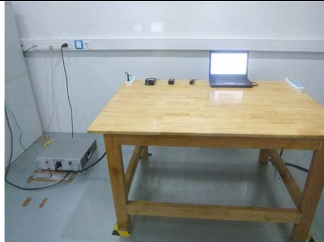
Conducted Emissions Test Setup Front View
