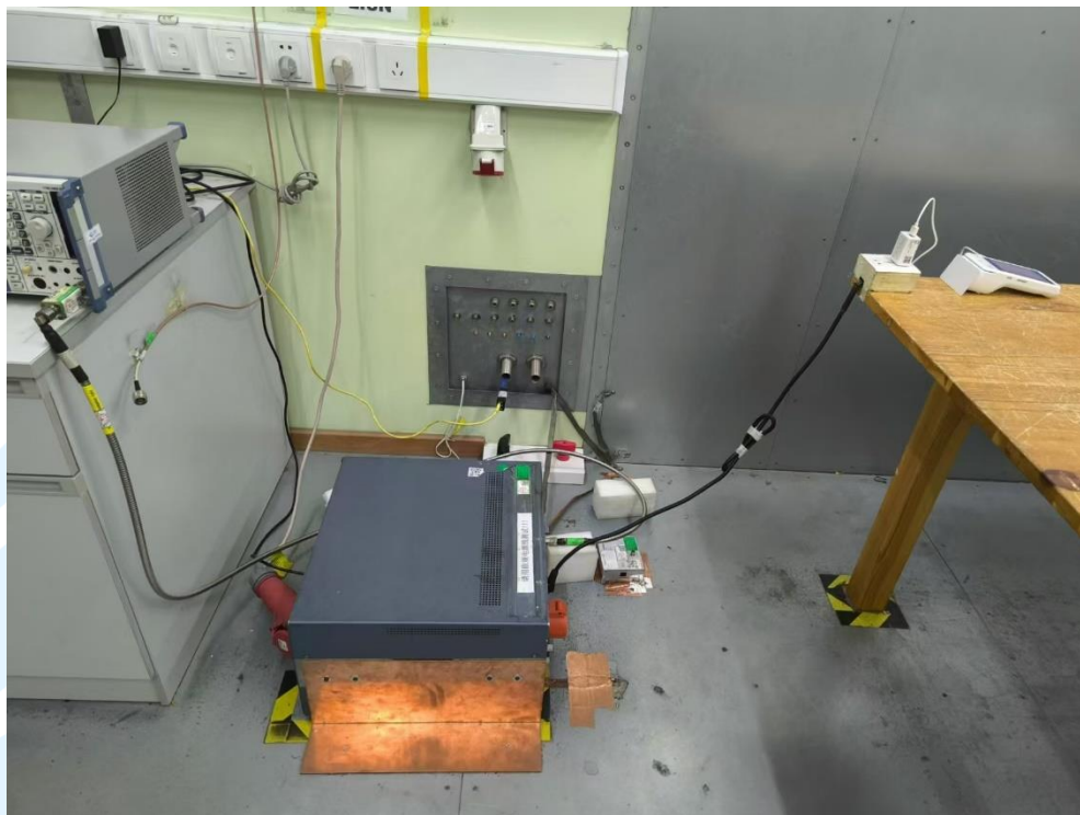
Conducted Emission Test Setup
