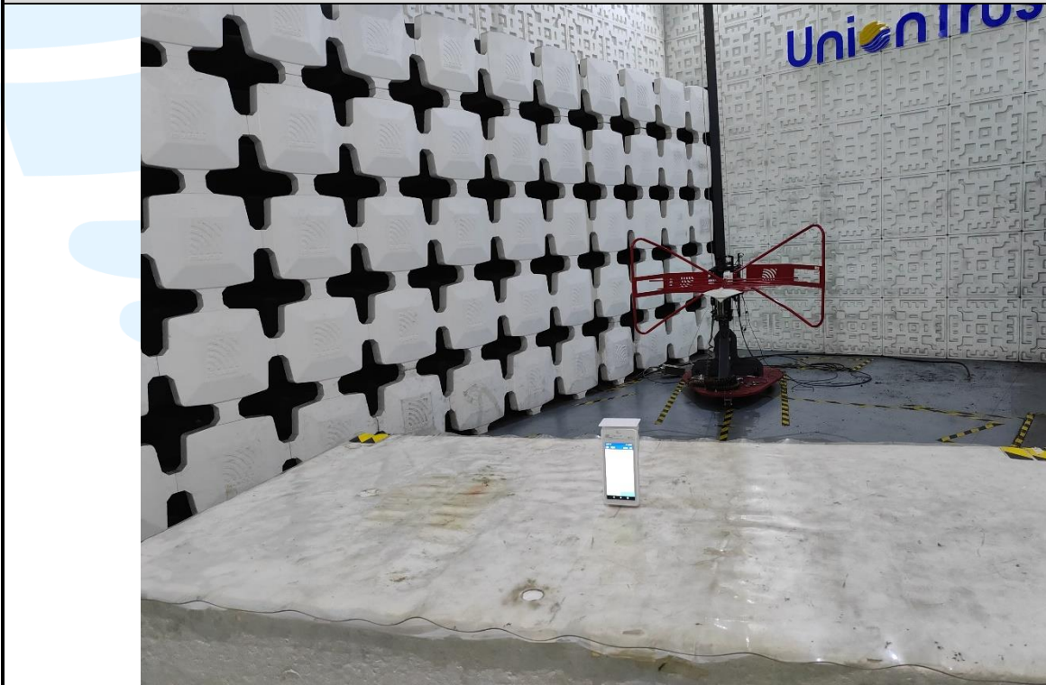
Radiated emission Test Setup (30 MHz~1 GHz)
