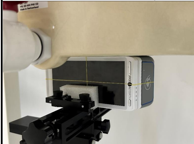
Left Side of EUT with 0 cm Gap
